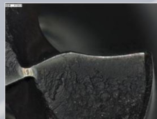
45m磨损图-HPD130
